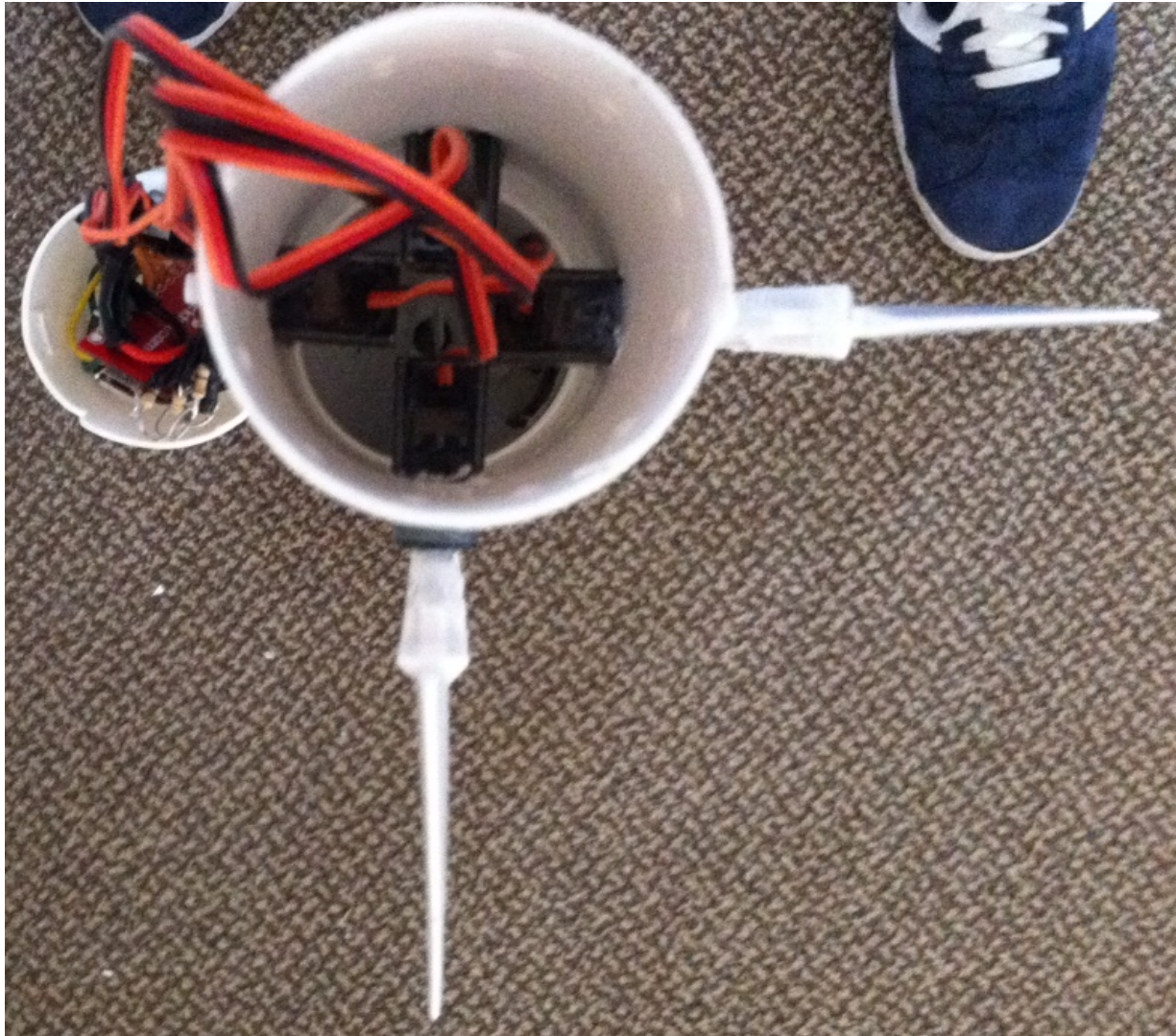
Figure 4. Servo Mounts. Four servos were mounted, level with each other. The horns stuck through the rocket body, where they were glued to nose fins. The nose fins are modified versions of the rocket's tail fins.
