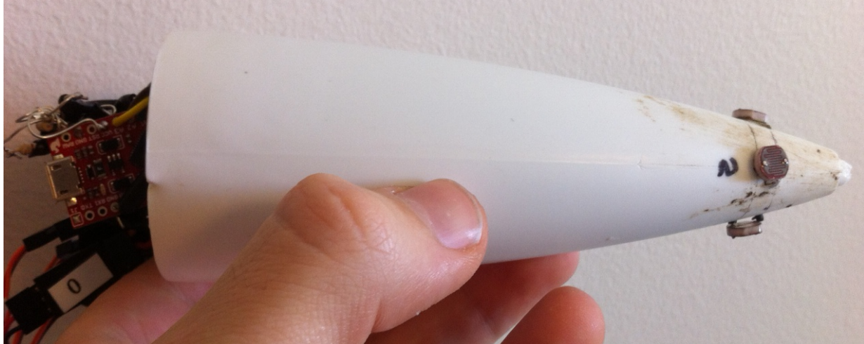
Figure 3. Sensor Tip. Four photoresistors are attached to the nose. Also shown, removable servo connectors, leading to the rest of the payload bay, which houses the actuators.
