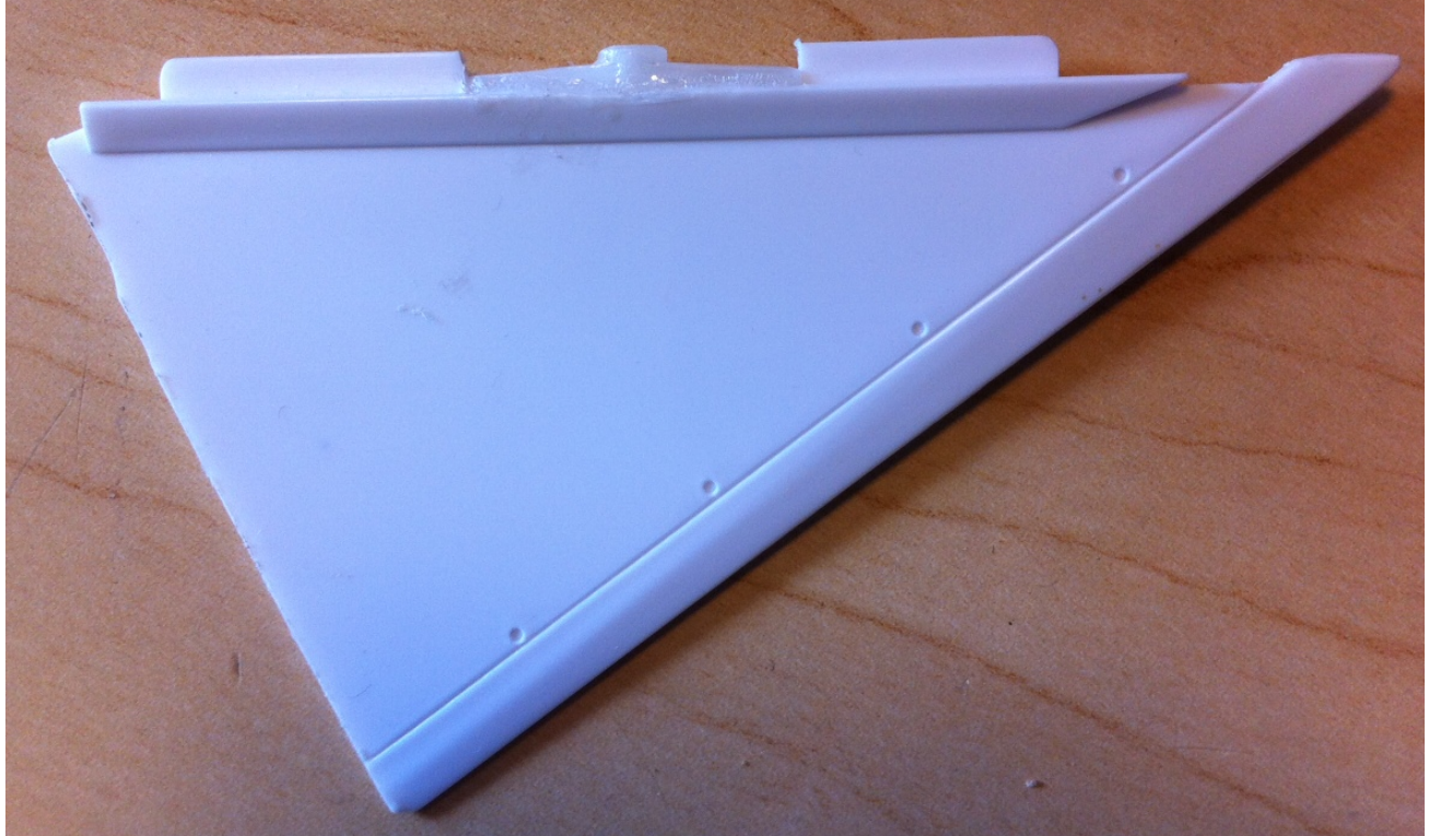
Figure 5. Rocket Nose Fin. The nose fins were built from the Estes Tomahawk's tail fins. Each fin was cut to reduce its area. The mount was also cut down and replaced with a servo horn, which snaps into a servo in the rocket body.
